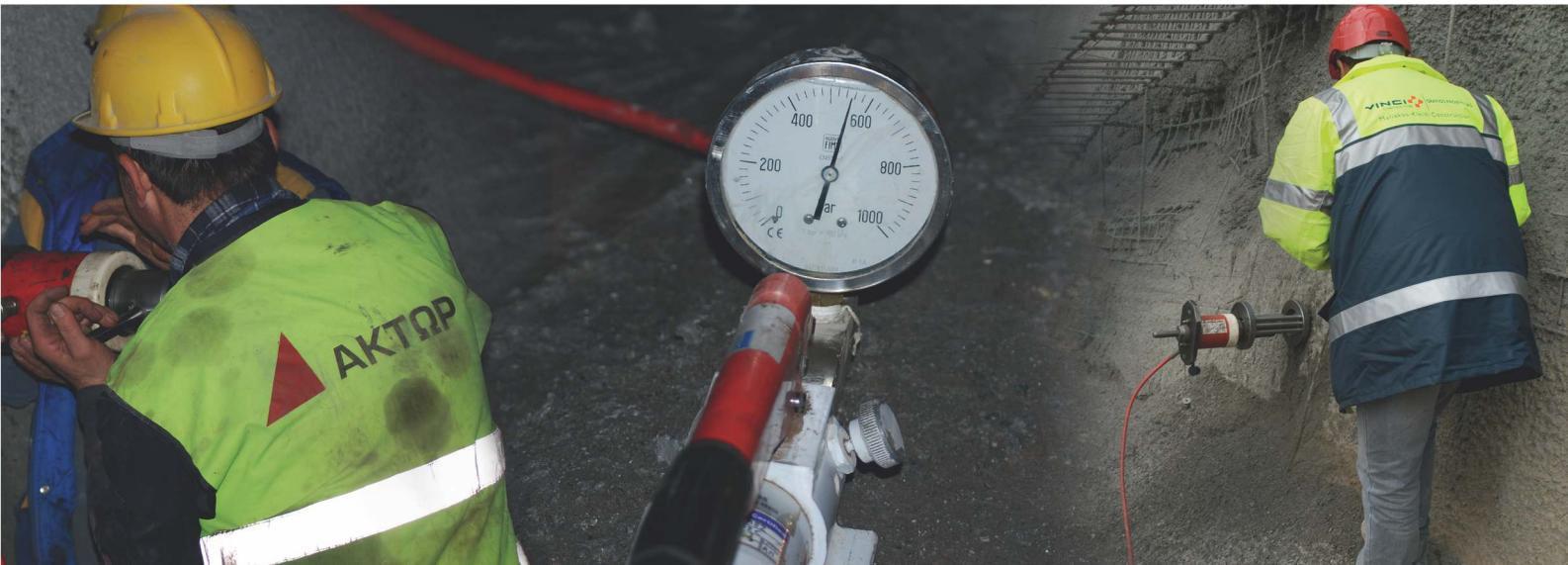
Complete pull-out test system for ELEBOLT™ friction bolts is available comprised of a hollow hydraulic cylinder, a hydraulic pump, a manometer for monitoring the applied load, a cylinder resting base and suitable gripping device.
